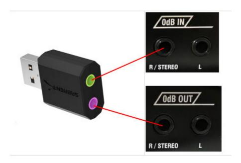
A possible connection between USB sound card and SEMPRA is shown here. **0db IN** and **0db OUT** are located on the back of the SEMPRA.
