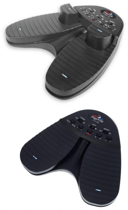
This foot switch - PageFlip Dragon - can be connected via Bluetooth as well as via USB. It is freely programmable via Bluetooth. If the footswitch is to be used only for turning pages, So the type - PageFlip Firefly - which can also be connected via Bluetooth is sufficient. The footswitches are also preprogrammed for AKcontrol and offered with the software.
