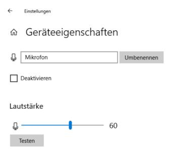
This setting only needs to be made once as we are connected to the 0db output of the organ. A value of 60 has proven to be beneficial in order to avoid overloading.
